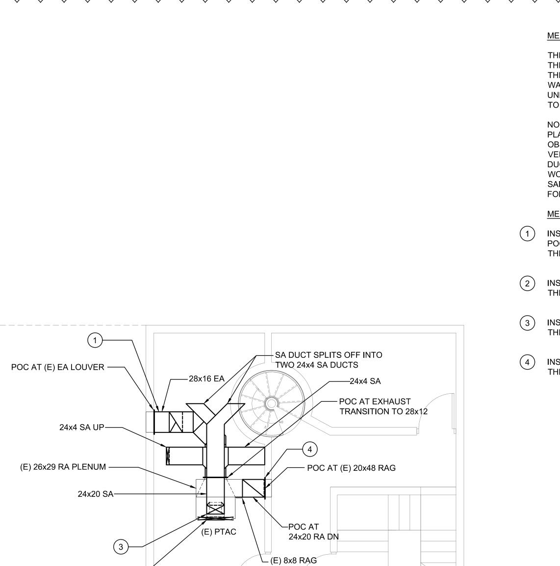
THE SCOPE OF WORK INVOLVES REPLACING THE EXISTING DUCTWORK CONNECTED TO THE PTAC UNIT. PORTIONS OF THE DUCTWORK WAS RECENTLY INSTALLED WHEN THE PTAC UNIT WAS REPLACED. THESE PORTIONS ARE TO REMAIN.
