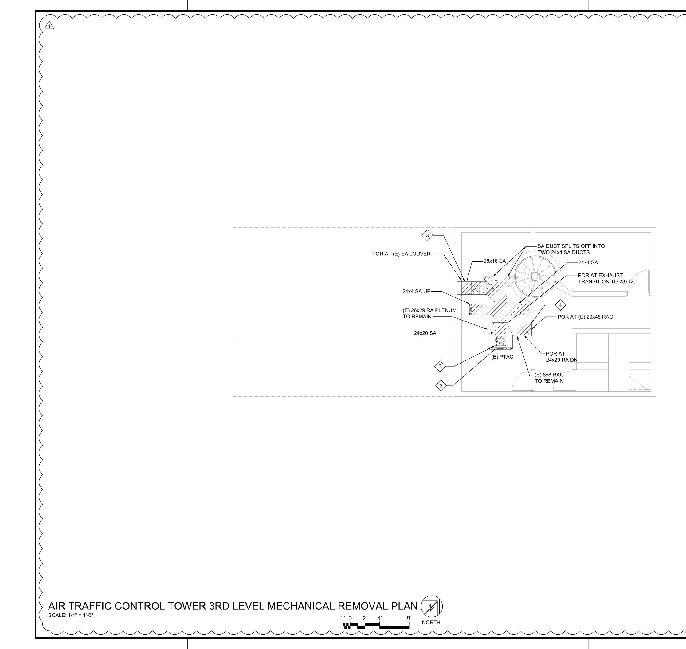
THE SCOPE OF WORK INVOLVES REPLACING THE EXISTING DUCTWORK CONNECTED TO THE PTAC UNIT. PORTIONS OF THE DUCTWORK WAS RECENTLY INSTALLED WHEN THE PTAC UNIT WAS REPLACED. THESE PORTIONS ARE TO REMAIN.
